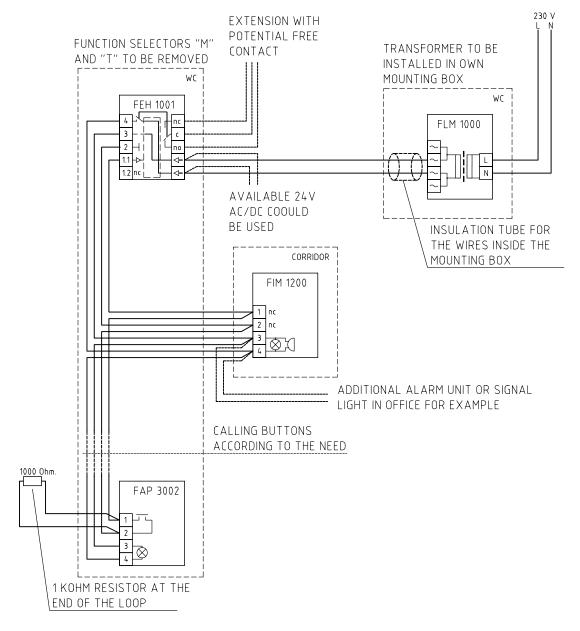
NOTE! WHEN NEEDED THE SUPPLY CIRCUIT INCLUDES A SWITCH WHICH DISCONNECTS ALL TERMINALS. THIS SWITCH MUST BE INSTALLED IN A PLACE WHERE UNINTENTIONAL USE IS PREVENTED
